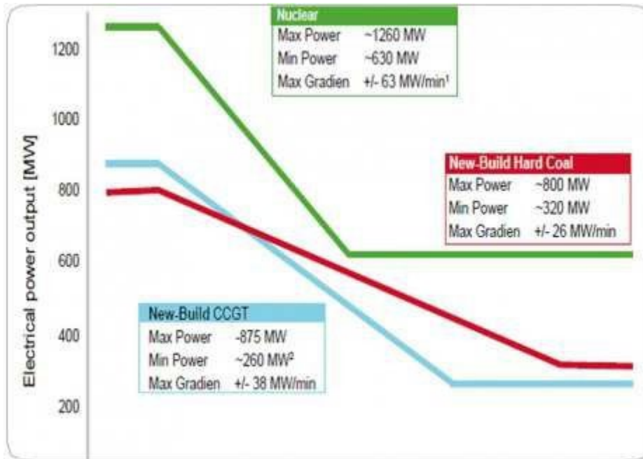
Figure 31 Comparison of load (power) response rates in different types of grid-connected power plants
