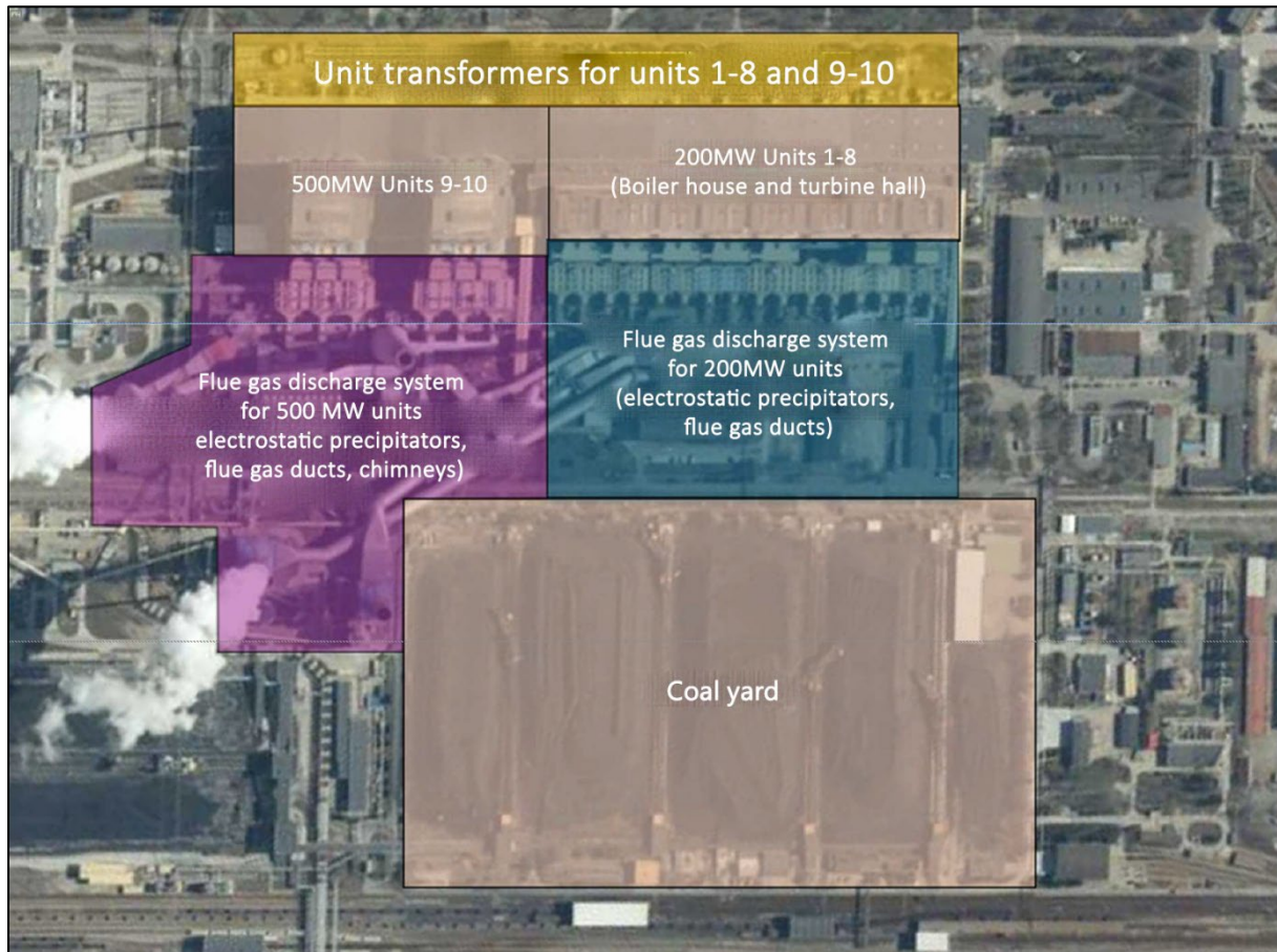
Figure 27 Location of the main power plant facilities
